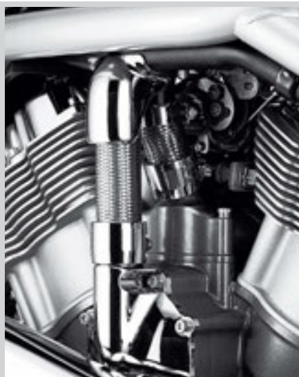
G. BRAIDED STAINLESS STEEL COOLANT LINE
