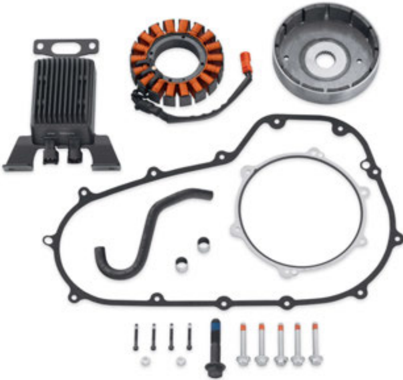
H. 54-AMP HIGH OUTPUT CHARGING SYSTEM
